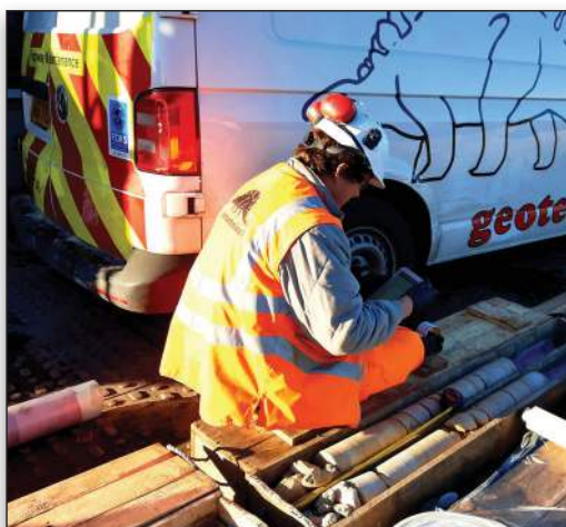
OpenGround Cloud data collector used on site to log rock core by Geotechnical Engineering Limited.
